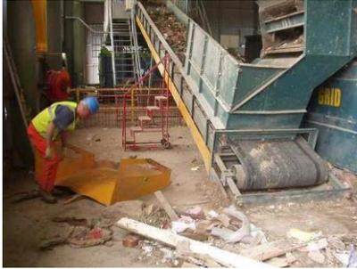
Bolted on 'fixed' guard removed from the end-run of a conveyor for maintenance at a construction waste recycling plant (this guard also has a padlock fitted to prevent unauthorised access)
