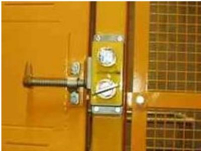
Retained key lock type interlock on an access gate to a machine enclosure – a key needs to be removed from the control box (stopping the machine) and inserted in the lock before the gate can be opened
