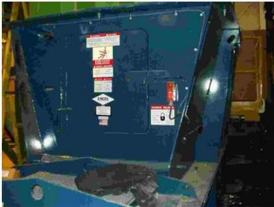
Hinged access door on baler to allow for blockage clearance protected by an interlock (the red box) on the access hatch. Some access hatches are also fitted with 'jailer's bars' inside the door or hatch to reduce the potential for access
